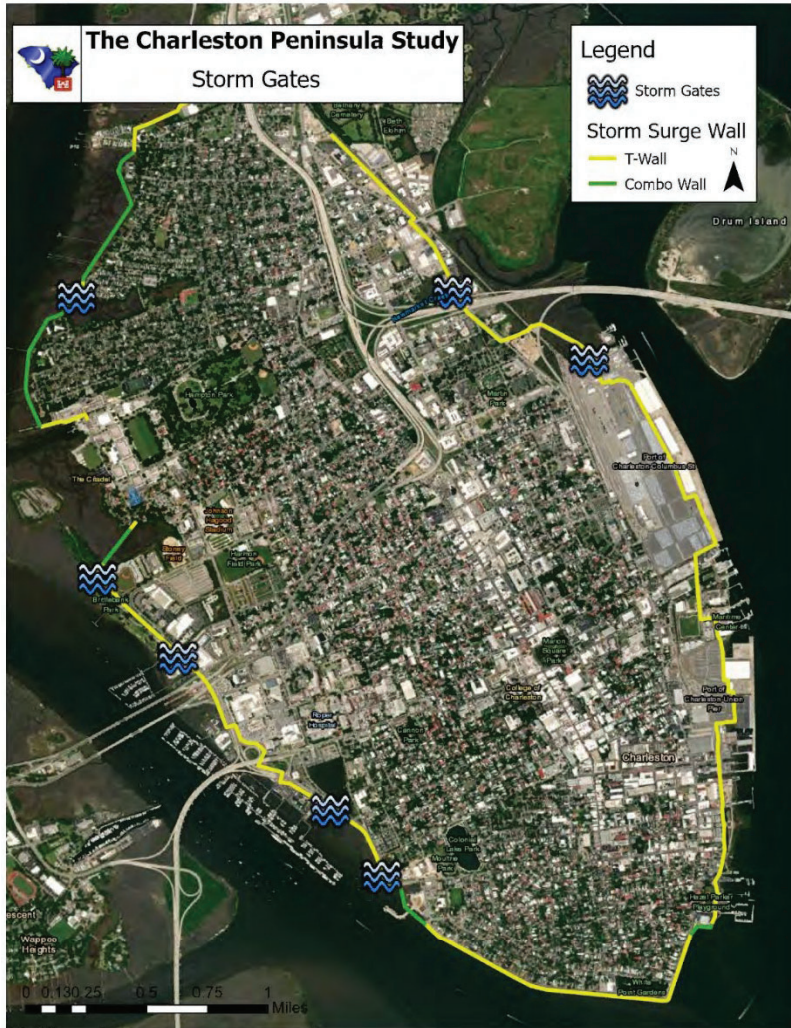
Map Showing Location of Storm Gates and Storm Surge Wall
