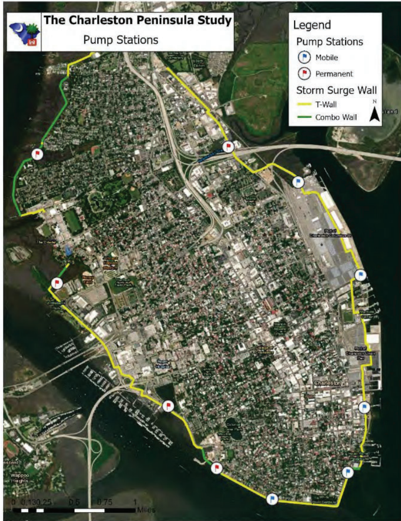
Map Showing the Locations of the Mobile (blue flags) and Permanent (red flags) Pump Stations
